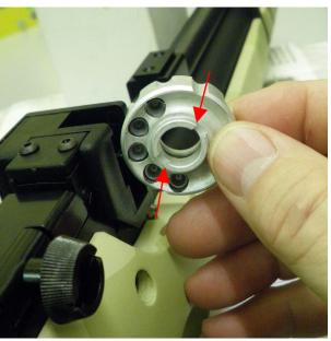
**Note:** To ensure the continued smooth operation of your magazine system, the pellet retaining O ring in the magazine needs to be regularly lubricated with a thin oil such as 3-in-1 to prevent premature wear and/or damage.
