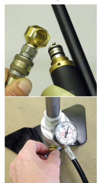
rifle is not cocked when the pump is used, the air will pass the valve and exhaust through the barrel.
