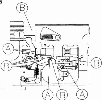
The wear parts of the Pro-Target have been designed to require minimal lubrication during normal use. The lubrication applied to the internal parts during assembly at the factory is normally sufficient for 10000 shots, any roughness of operation may indicate that lubrication is necessary before this number.
