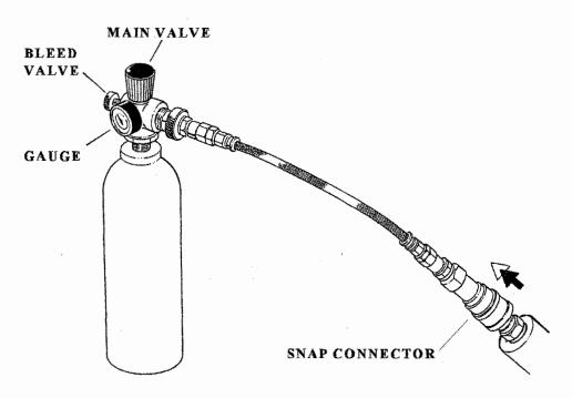
**NOTE!** - If the rifle is empty of air it must be cocked prior to filling. Air will exhaust from the barrel if this is not done.
