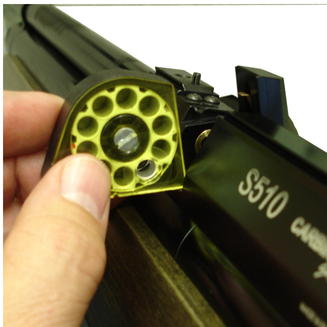
Pinch the magazine out of the housing
