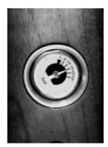
This picture shows a guns with just over 150 bar of pressure. Although every gun is slightly different the recommended refill pressure for the S400 is between 100 and 110 bar.
