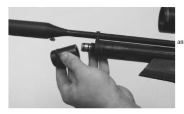
This is achieved by unscrewing the cover in an anti-clockwise direction.
