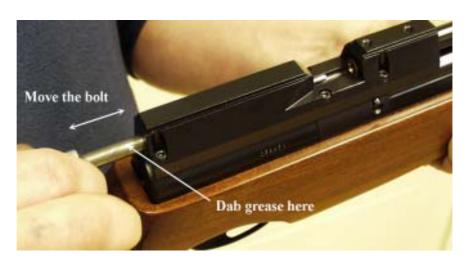
APPLY A SMALL DAB OF GREASE ON THE LOADING BOLT AND WORK-IN BY MOVING THE BOLT FORWARDS AND BACKWARDS. WIPE OFF EXCESSIVE GREASE ASE, FREFERRED GREASE IS 'NAPIER G95 GUN GREASE'
