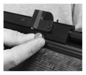
On the left side of the rifle is an indicator to help select your power setting. + = High, - = Low. The marks do not indicate a particular power as this would change depending on the pellets used.
