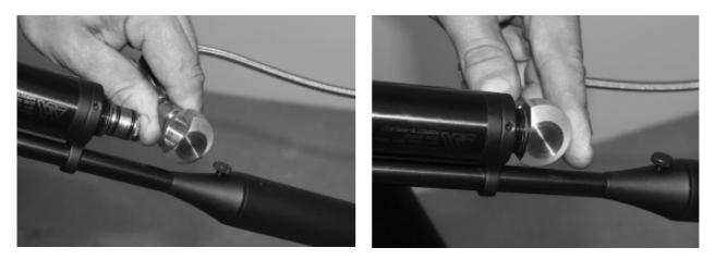
It is a wise precaution to hold the female part of the connector, during the filling procedure, as shown in the pictures below. This will ensure the female adaptor is located completely over the male part and prevent any accidental dislodging of the connector before you start to refill the cylinder.
